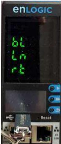
6. The update should take about a minute. Then the controller will reboot. The LCD display will go back to displaying power data and show the colored LED border. After another minute you will see the LED display show the Enlogic logo and boot up progress indicator.
